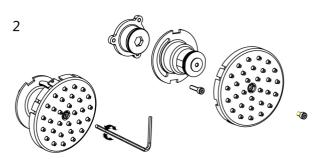
Remove the M4X12 screw and the outlet face Remove the M4X20 screw and the connector body
